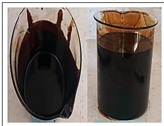
Figure 2. Stable water-in-oil emulsions (70:30 v/v% crude to brine water) for KD1 (right) and DGH2 (left), after 3-h settling time.
